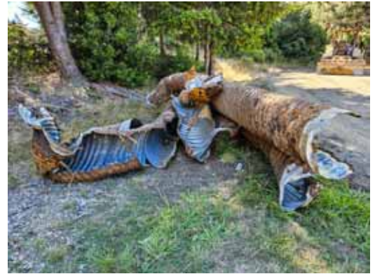
The paving repair at the NFS uncovered some seriously degraded underground culverts! They have been replaced with much-improved versions.
